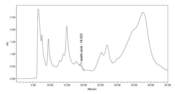
FIGURE 5. HPLC analysis for acetic acid in CPA-PB
