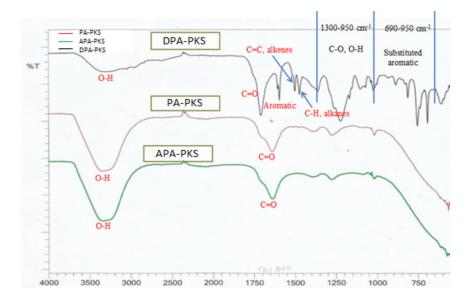
FIGURE 3. FTIR spectrum of DPA-PKS, PA-PKS and APA-PKS
