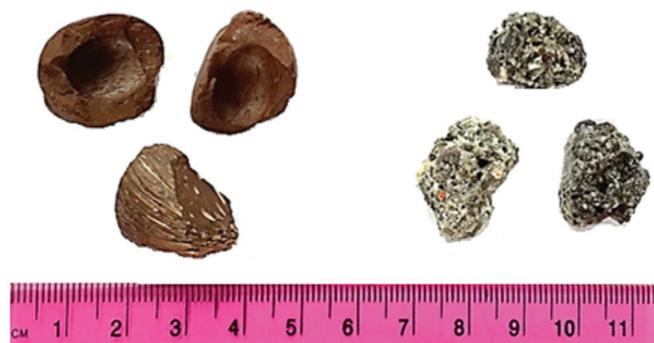
FIGURE 1. Oil palm shell (left) and oil-palm-boiler clinker (right)
