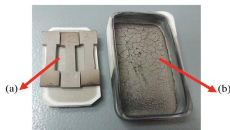
FIGURE 7. Physical deformation after sintering temperature at 1100°C (a) Ti-6Al-4V/HA with NaCl (b) Ti-6Al-4V/HA with PMMA
