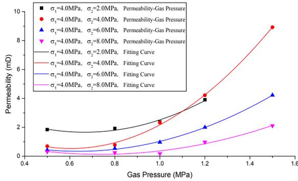
FIGURE 5. Fitted curve of permeability versus gas pressure
