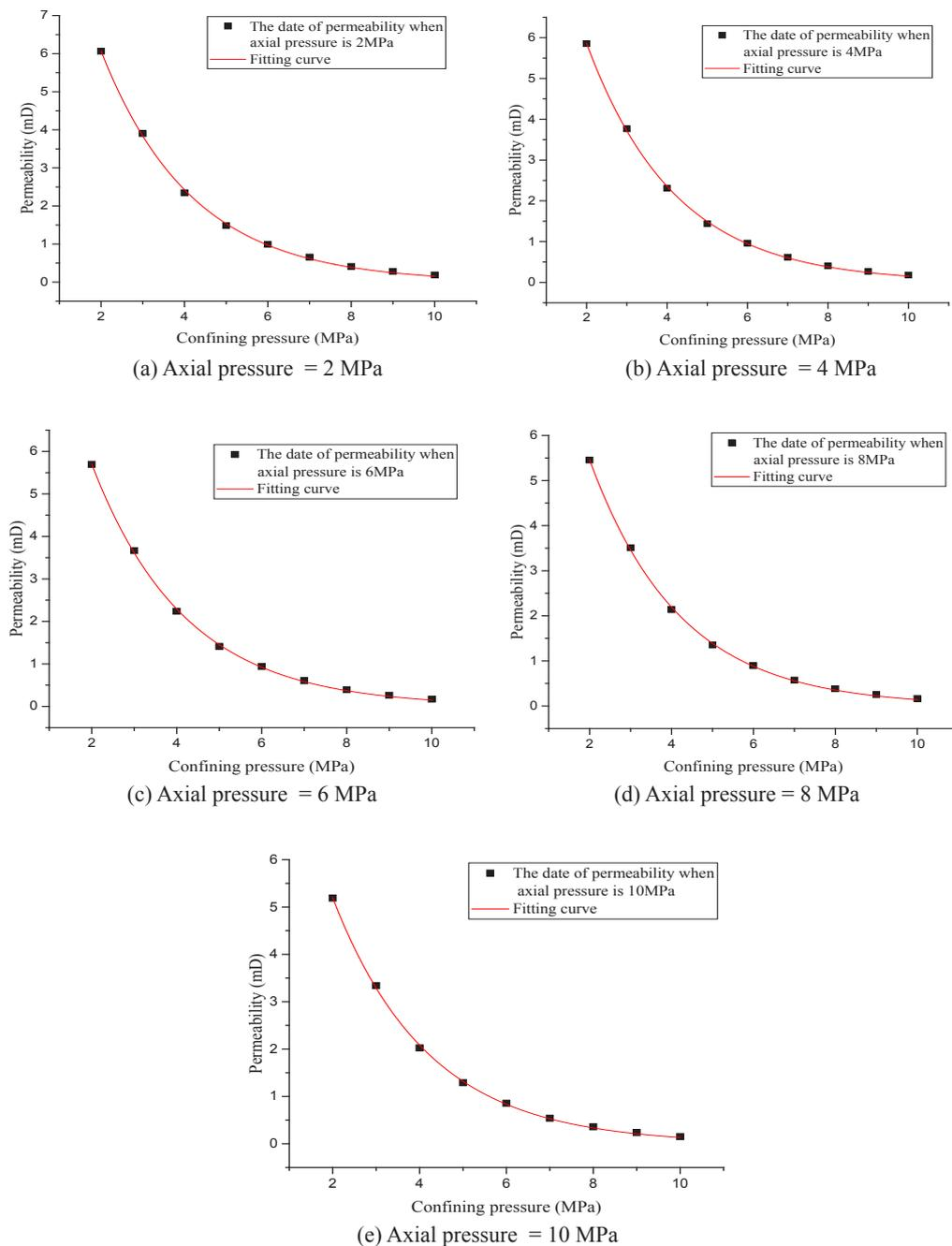
FIGURE 2. Permeability versus confining pressure at 2–10 MPa axial pressure ( $\sigma_1$ )
