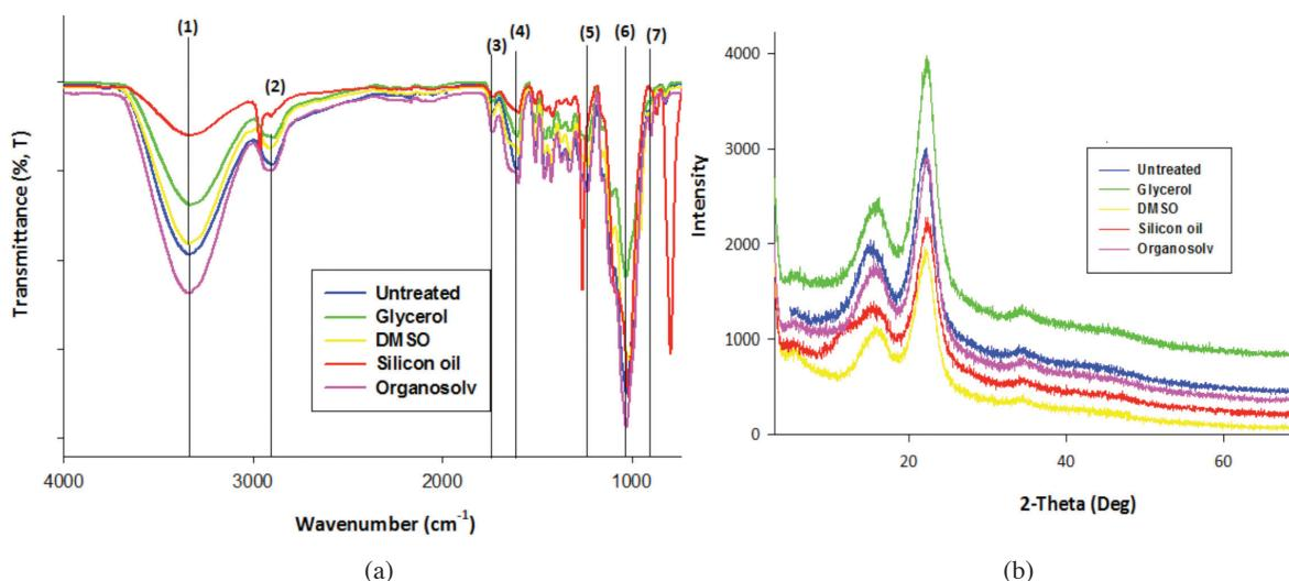
FIGURE 2. (a) ATR-FTIR spectral analysis of untreated *kempas* and treated *kempas* in glycerol, DMSO, silicon oil and organosolv. FTIR spectra bands (cm<sup>-1</sup>): (1) 3349 cm<sup>-1</sup>; (2) 2902 cm<sup>-1</sup>; (3) 1731 cm<sup>-1</sup>; (4) 1597 cm<sup>-1</sup>; (5) 1235 cm<sup>-1</sup>; (6) 1029 cm<sup>-1</sup>; (7) 895 cm<sup>-1</sup>(amorphous) and (b) XRD analysis of untreated and pretreated *kempas* in glycerol, DMSO, silicon oil and organosolv (ethanol/water)
