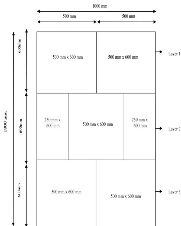
FIGURE 1. Schematic diagram of wall type A
