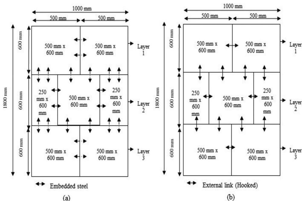
FIGURE 2. Schematic diagram of wall B with internal link (embedded) (a) and external link (hooked) (b)
