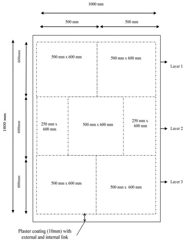
FIGURE 3. Schematic diagram of wall type C &amp; D
