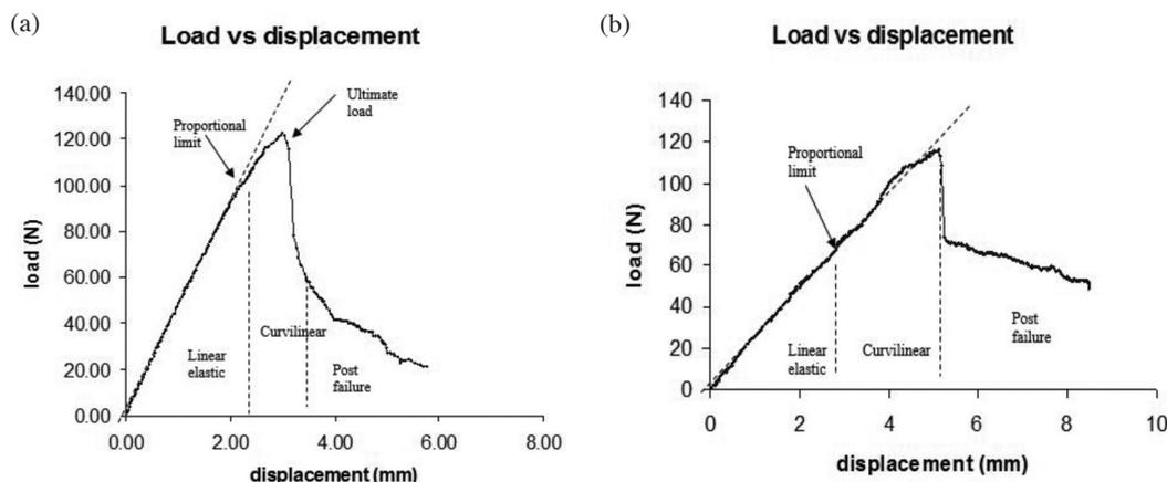
FIGURE 4. Load versus displacement of bending test for (a) 50 mm wood wool cement board and (b) 75 mm wood wool cement board
