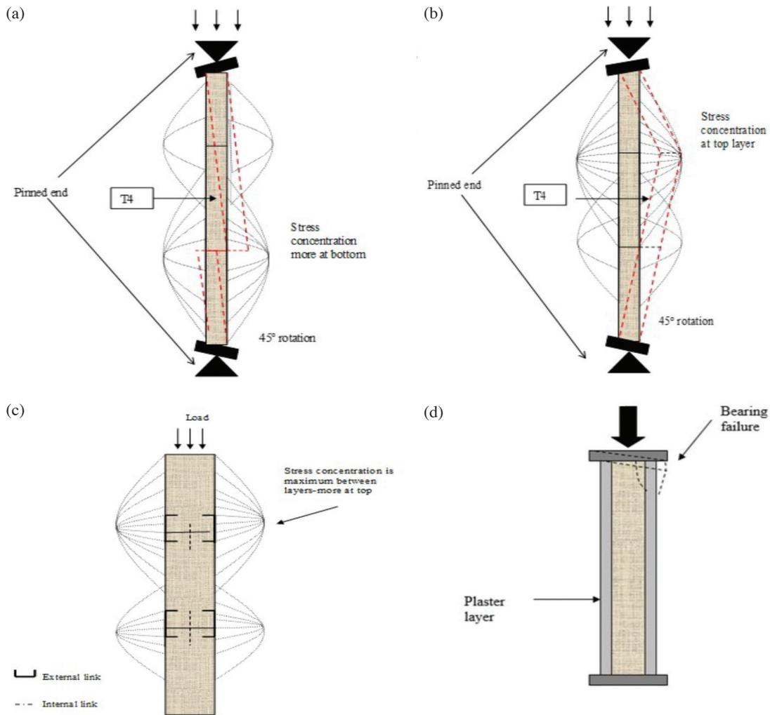
FIGURE 5. Schematic diagram of failure mode for walls produced: (a) wall A1, (b) wall A2, (c) wall B and (d) wall C & D
