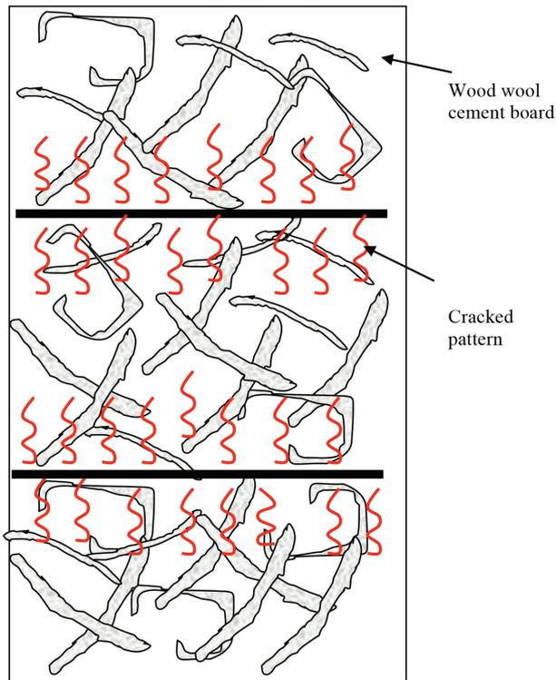
FIGURE 7. Cracked pattern at the surface for wall B1 and B2
