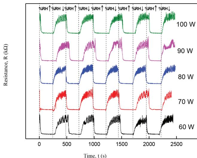
FIGURE 4. Dynamic response of the a-CN<sub>x</sub> thin films deposited at different RF power to different RH levels, 4-87%
