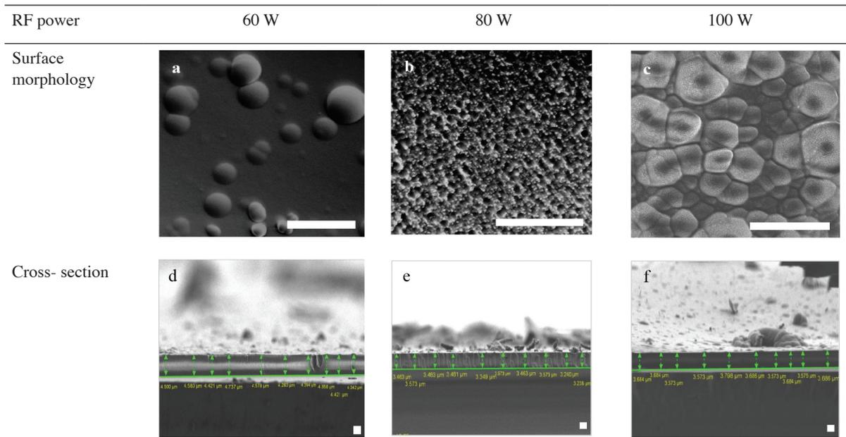
The scale bar shown for 2  $\mu\text{m}$
