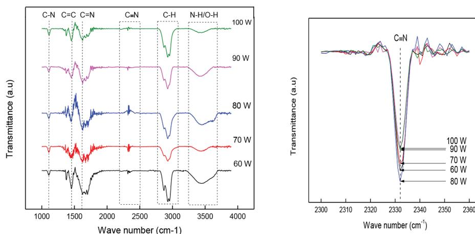
FIGURE 3. (a) Variation in FTIR transmittance spectra for films deposited as a function of RF power, (b) spectra of a specific region near 2330 cm<sup>-1</sup> for the formation of triple bond (C≡N)
