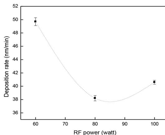
FIGURE 2. Deposition rate variation with RF power for a-CN<sub>x</sub> thin films
