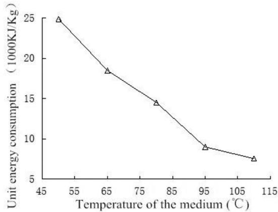
FIGURE 6. Variation of heat consumption per unit
