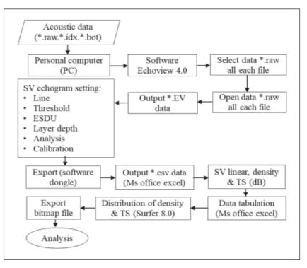
Fig. 2. Flowchart of processing and analysis of acoustic data.
