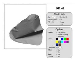
Figure 1: Optical scan (EinScan-Pro Scan, 3D Systems) of right orbital implant in stereolithographic (STL) data
