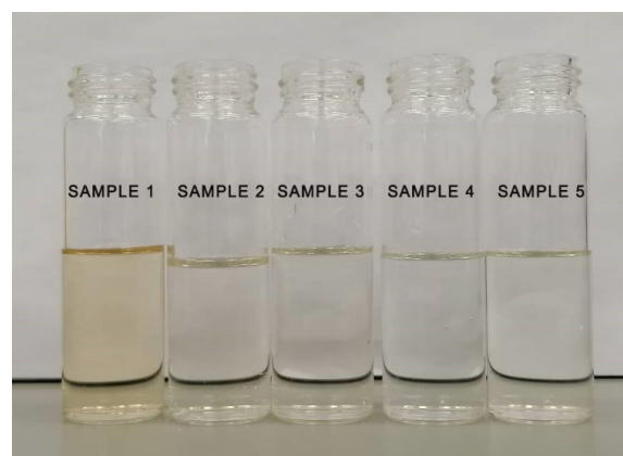
FIGURE 6. Rejection and the collection of permeates of humic acid after filtration of all samples
