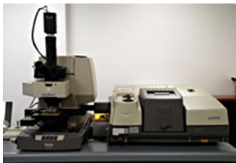
FIGURE 2. FTIR machine (Nicolet 6700 machine)
