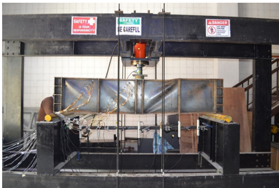
FIGURE 4. Formation of diagonal buckling in typical web panels
