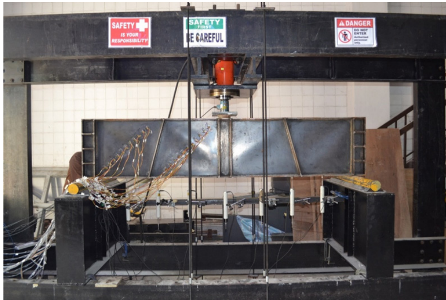
FIGURE 4. Formation of diagonal buckling in typical web panels
