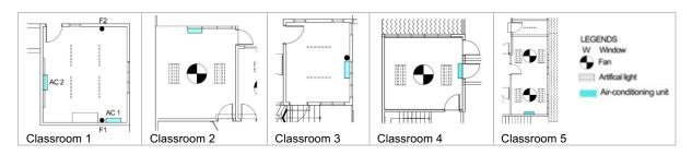
Figure 10: Location of Air conditioning unit and fan in classroom 1, 2, 3, 4 and 5.
