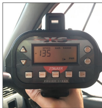
FIGURE 2. Radar gun showing the measurement of spot speed
