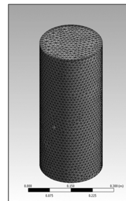
FIGURE 9. Mesh structure of 3D FBD model.
