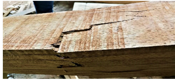
Figure 5. Cracks due to failure of glulam under flexural testing
