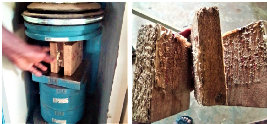
Figure 3. (a) Prepared shear block for the test; (b) Failure and delamination of adhesive on the specimen
