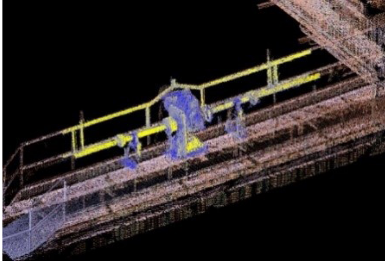
FIGURE 8. Registered hydraulic pump of registered point clouds from handheld scanner into point clouds from TLS
