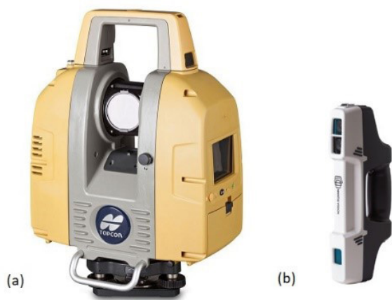
FIGURE 2. (a) TLS Topcon GLS-2000 (source: www.topcon.com); (b) HLS Stonex F6 (source: www.mantis-vision.com)
