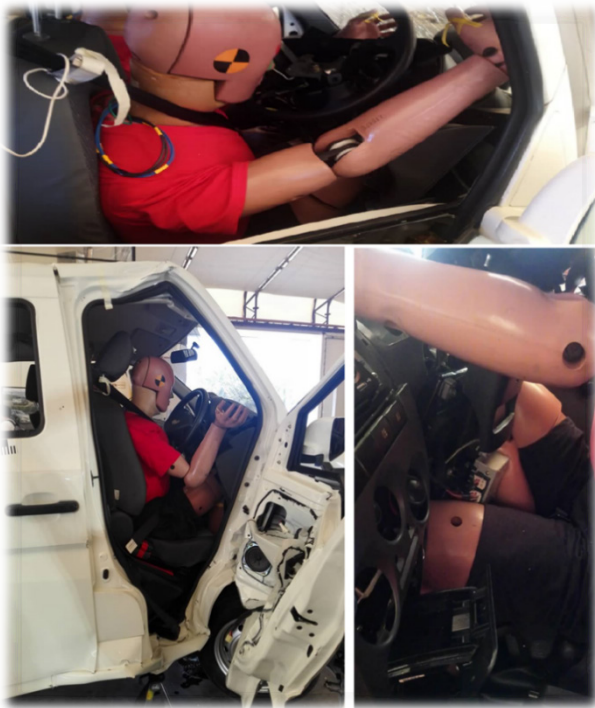
FIGURE 6. ASEAN NCAP's panel van; dummy injury in frontal offset crash test
