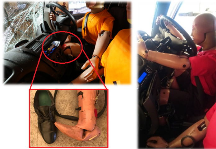
FIGURE 5. ASEAN NCAP's small lorry dummy injury in frontal offset crash test
