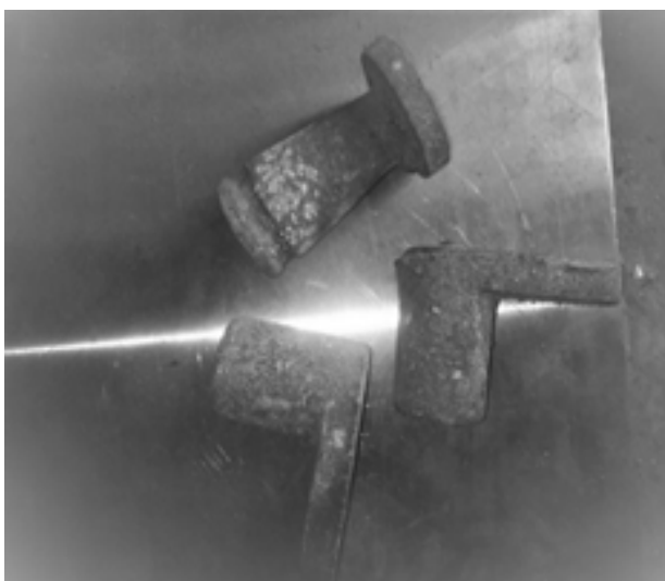
FIGURE 7. Ceiling Fan Winding Machine Components (a) Cast Iron (b) Steel
