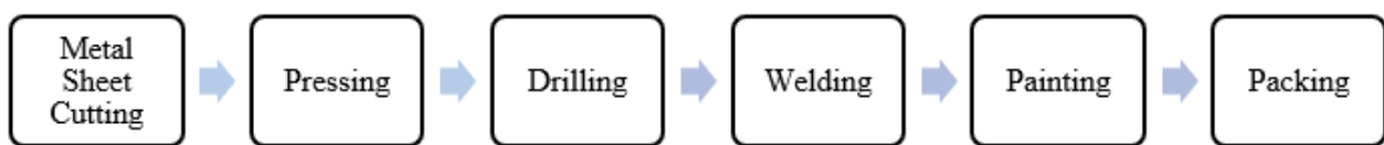
FIGURE 6. Ceiling Fan Winding Machine Manufacturing Process
