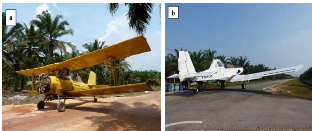
Figure 1. Type of agricultural aircraft used for the Bt aerial spraying, (a) Grumman G-164 A Super AgCat, (b) Mielec M-18 Dromader
