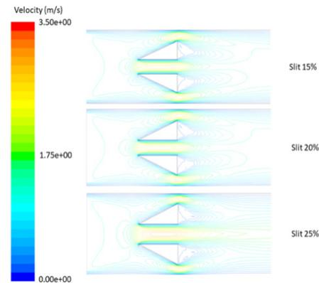
FIGURE 4. Velocity contour at slit gap 15%, 20% and 25%
