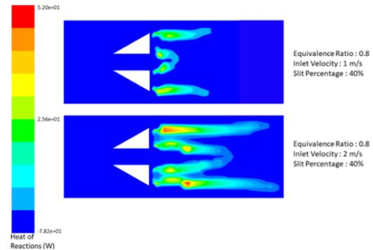
FIGURE 3. Contour heat of reaction at inlet velocity 1 m/s and 2 m/s
