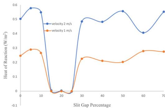
FIGURE 2. Heat reaction at various slit gap
