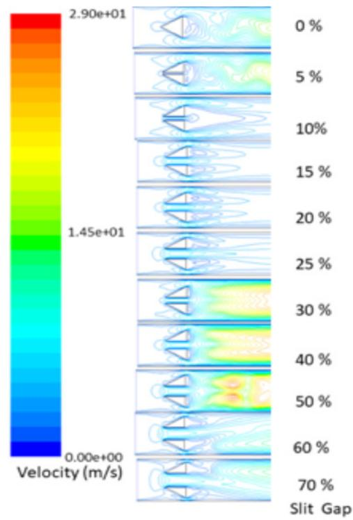
FIGURE 5. Velocity contour at various slit gap
