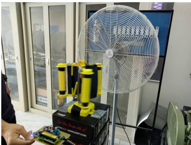
FIGURE 6. Test set up for the Magnus wind turbine
