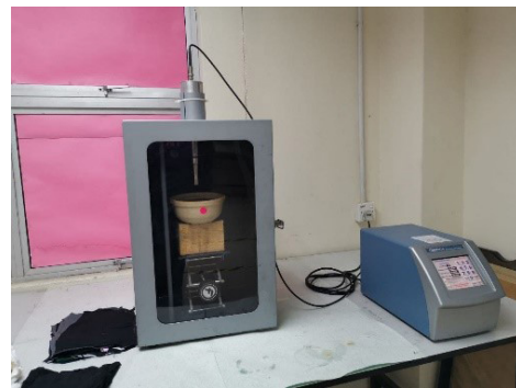
FIGURE 3. Sonicator set up to prepared nano medium
