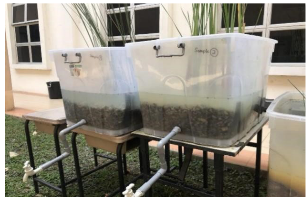
FIGURE 1. The pilot-scale of constructed wetland using HSF and VSF with Typha Angustifolia
