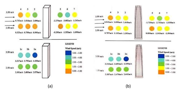
Figure 7: (a) Wind flow pattern of square prism model; above: wind flow from windward to leeward, below: wind flow from side surface; (b) Wind flow pattern of Gran Torre Santiago model; above: wind flow from windward to leeward, below: wind flow from side surface
