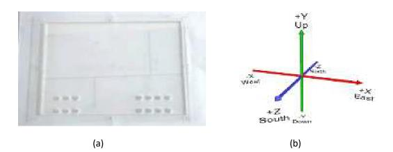
Figure 5: (a) Total of 14 traverse points on the cover of testing section; (b) Axis of traverse points
