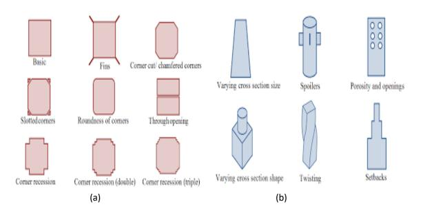
Figure 2: (a) Minor aerodynamic modifications; (b) Major aerodynamic modifications (Power & Jayachandran, 2019)
