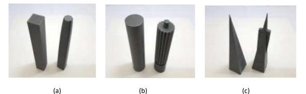
Figure 3: (a) Square geometry and duplicated model of Gran Torre Santiago; (b) Cylinder geometry and duplicated model of Marina City Towers; (c) Pyramidal geometry and duplicated model of Transamerica
