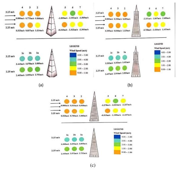
Figure 9: (a) Wind flow pattern of pyramidal model; above: wind flow from windward to leeward, below: wind flow from side surface; (b) Wind flow pattern of Transamerica model (section X); above: wind flow from windward to leeward, below: wind flow from side surface; (c) Wind flow pattern of Transamerica model (section Y); above: wind flow from windward to leeward, below: wind flow from side surface
