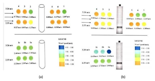
Figure 8: (a) Wind flow pattern of cylindrical model; above: wind flow from windward to leeward, below: wind flow from side surface; (b) Wind flow pattern of Marina City Tower model; above: wind flow from windward to leeward, below: wind flow from side surface
