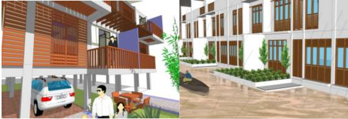
Figure 1 Contemporary terrace houses with pilotis element provide spaces for multi-purpose and control of flood disaster.
