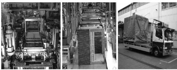
Figure 1: The process of manufacturing and delivery of volumetric IBS in the Sekisui Heim factory
