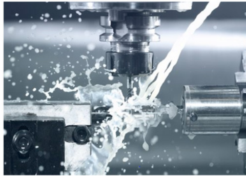
FIGURE 3. The use of cutting fluid for steel projects (Wasatch steel cutting, 2021)
