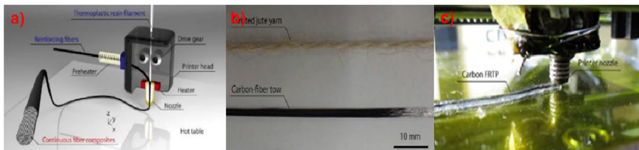
FIGURE 1. (a) Schematic of the 3D printer head used to produce continuous fibre reinforced thermoplastics using in-nozzle impregnation based on FDM, (b) the thermoplastic resin filament and reinforcing fibres are sent to printer head separately, (c) continuous carbon fibre-reinforced composites are manufactured using a 3D printing process (Matsuzaki et al. 2016).
