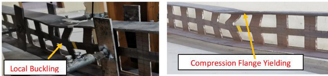
d) Local highly distorted web - flanges and web for SSB
