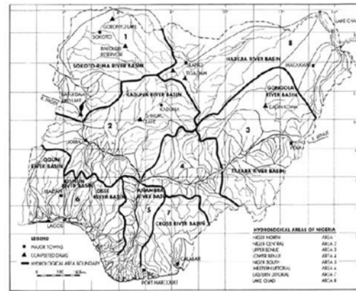
FIGURE 2. Hydrological map of Nigeria showing the large dams and their locations in their respective river basins (Akindele, and Indabawa, 2015).
