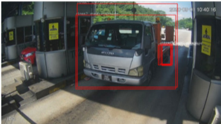
FIGURE 3. Redundant detection occurs in practical situation.
