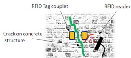
FIGURE 18. RFID reader wirelessly interrogates a couplet of RFID tags that were placed on the cracked wall (Caizzone & DiGiampaolo 2015)
