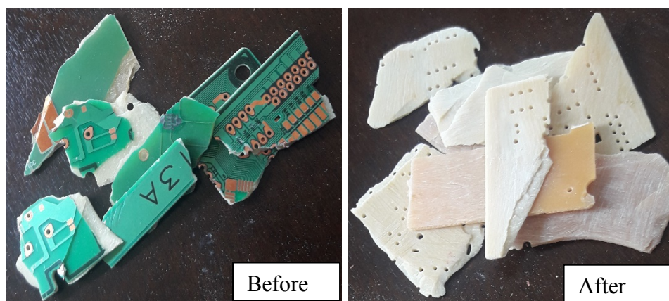
FIGURE 1 Image of NMPCB before and after the removal of copper layer
