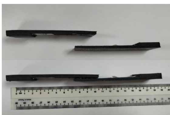
FIGURE 3. Unbonded half of single lap shear test specimen with extra tab printed and final geometry of specimen after bonding.
