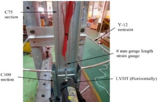
(b) Strain gauge and LVDT (Horizontal direction) position
