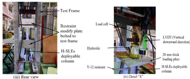
(c) Views of isolated H-SLEs deployable column under load test configuration
