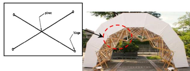
FIGURE 1. Scissor-like elements (SLEs) mechanism for deployable structure application
