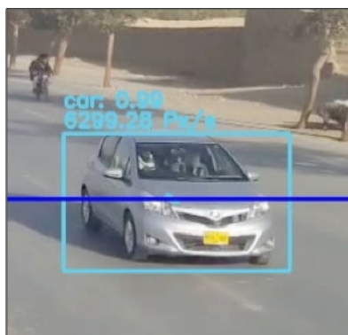
FIGURE 3. A detected car with speed in pixels per second, with 99% confidence
