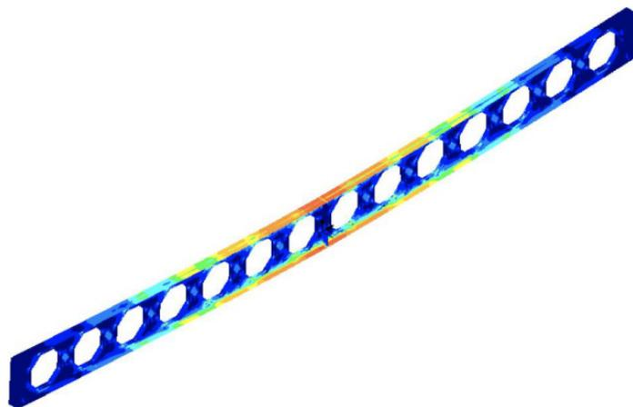
FIGURE 13. Stress concentration in a typical castellated beam CB 11500
