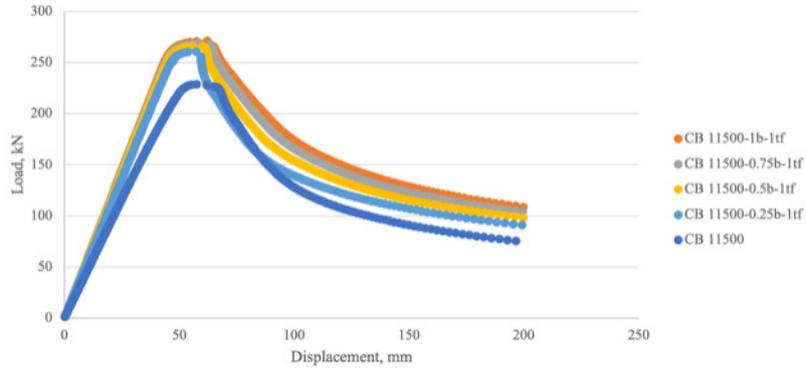
FIGURE 14. Load-displacement relationship of castellated beams CB 11500 (effects of stiffener width)
