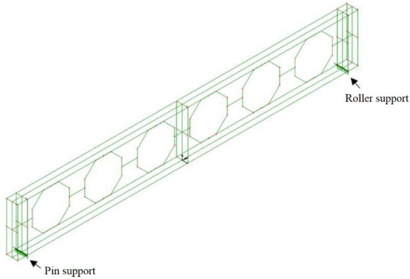
FIGURE 4. Assignment of boundary conditions
