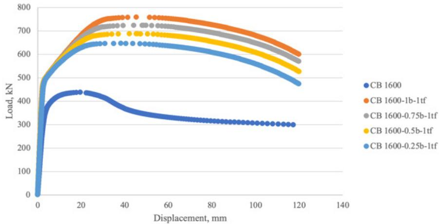
FIGURE 9. Load-displacement relationship of castellated beams CB 1600 (effects of stiffener width)
