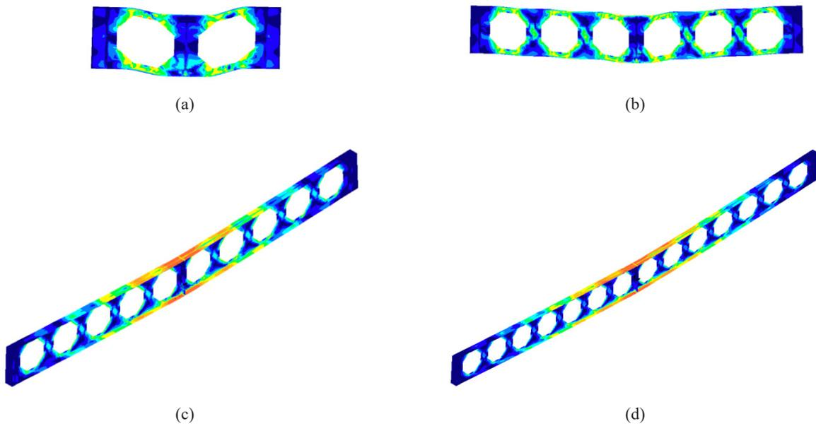
FIGURE 8. Stress contour in castellated beams; (a) CB 1600, (b) CB 5000, (c) CB 8200 (d) CB 11500
