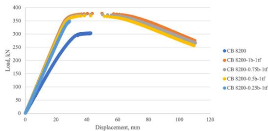
FIGURE 12. Load-displacement relationship of castellated beams CB 8200 (effects of stiffener width)
