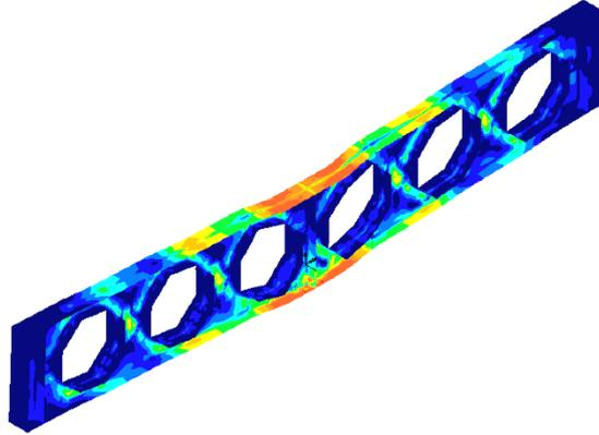
FIGURE 11. Stress concentration in a typical castellated beam CB 5000
