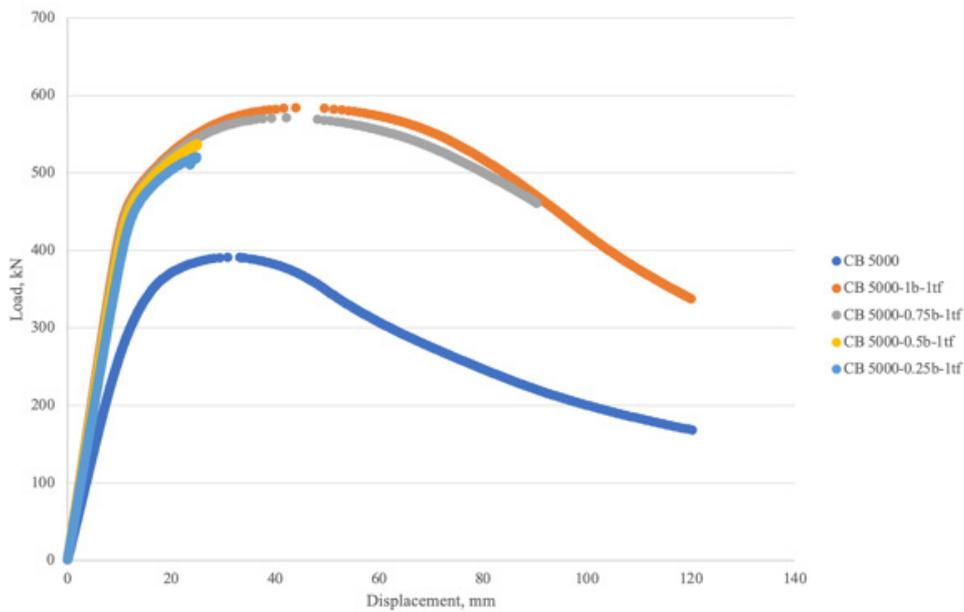
FIGURE 10. Load-displacement relationship of castellated beams CB 5000 (effects of stiffener width)
