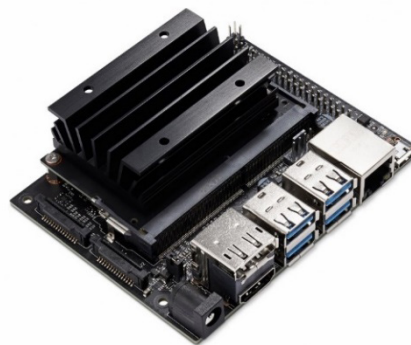
FIGURE 1. Nvidia Jetson Nano single board computer with 128 CUDA or 128 GPU cores to perform large data processing in deep learning.
