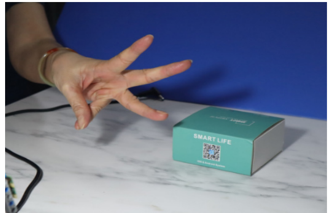
FIGURE 7. Improper staging of the hand position away from the small platform may cause error in classification due to image out of frame.
