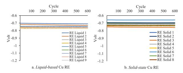
FIGURE 6. OCP value by 10 sample of (a) Liquid-based Cu and (b) Solid-state Cu RE
