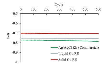
FIGURE 8. Validation Stability of OCP test by Solid-state Cu RE, Liquid-based Cu RE vs Ag/AgCl Commercial Reference Electrode
