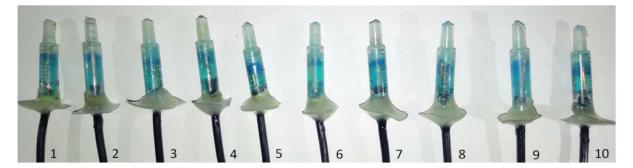
FIGURE 3. 10 sample liquid-based Cu/CuSO<sub>4</sub> reference electrode
