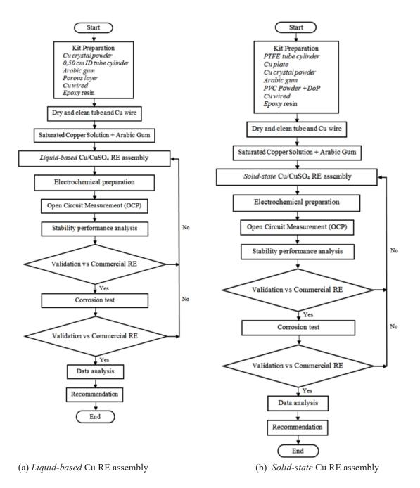
FIGURE 1. Flow chart Liquid-based and Solid-state Reference Electrode assembly
