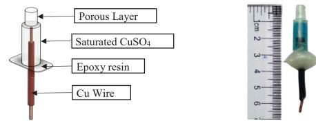
(a) Desain liquid-based Cu Reference Eelctrode
