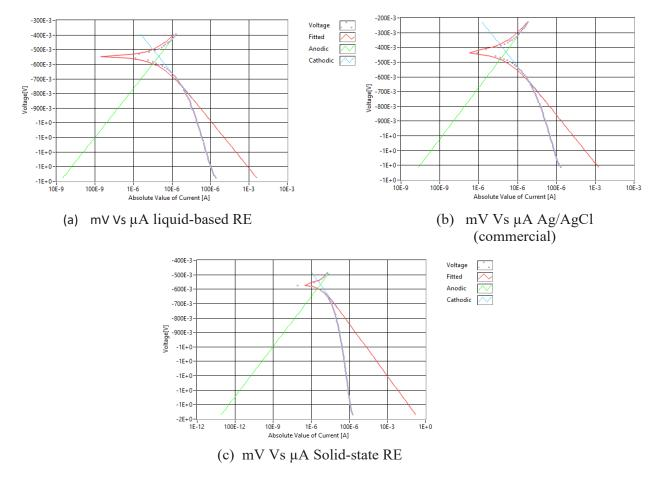
FIGURE 9. Ecorr and Icorr Reference Electrode analysis
