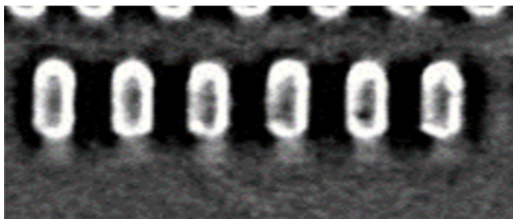
FIGURE 11. X-ray laminography of lead with Sn plating 5 \mu\text{m}
