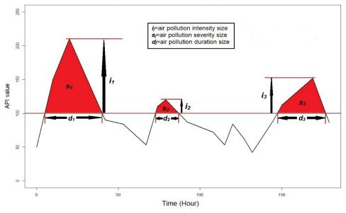
FIGURE 3. Air pollution characteristics based on their duration, intensity, and severity
