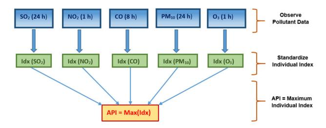
FIGURE 2. Process of determining the API value
