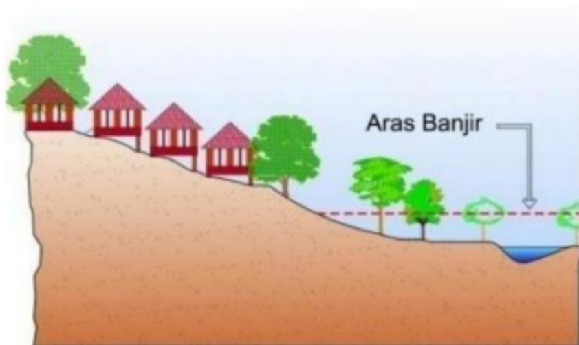
FIGURE 4. Development that uses the zoning control method in the floodplain channel zone. Source: KSAS Conservation and Development Planning Guidelines, 2017
