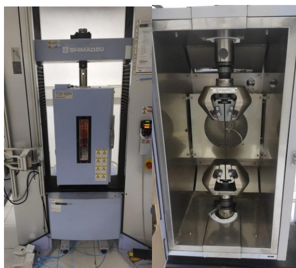
FIGURE 4. (a) Shimadzu AG-50KNX UTM Machine with TCE-N300 Thermal Chamber (b) Inside of TCE-N300 Thermal Chamber
