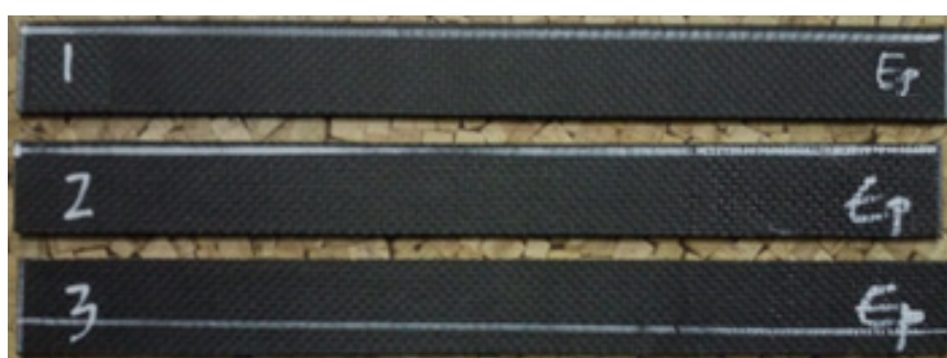
FIGURE 5. Carbon/LY5052 composite specimens from the vacuum infusion process
