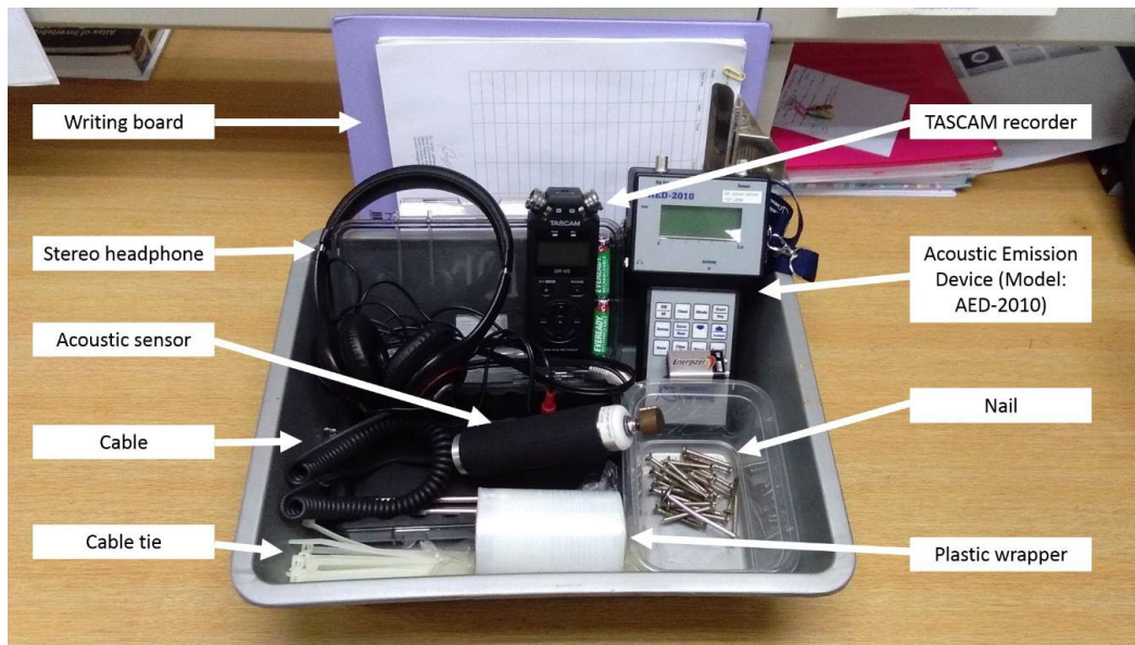
Figure 2. Acoustic recording equipment, model AED 2010
