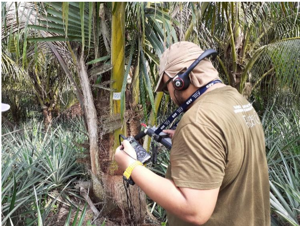
Figure 3. Acoustic recording of RPW at the infested coconut trees
