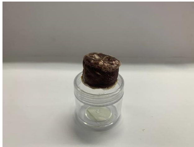
RAJAH 1(b). Aerogel PVA/2%MCC selepas proses silanisasi
