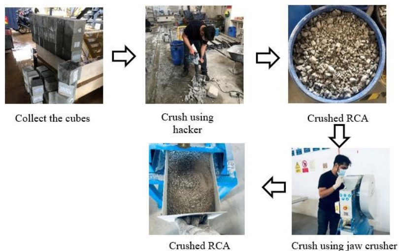
FIGURE 2. Process of the preparation of the recycled concrete aggregate
