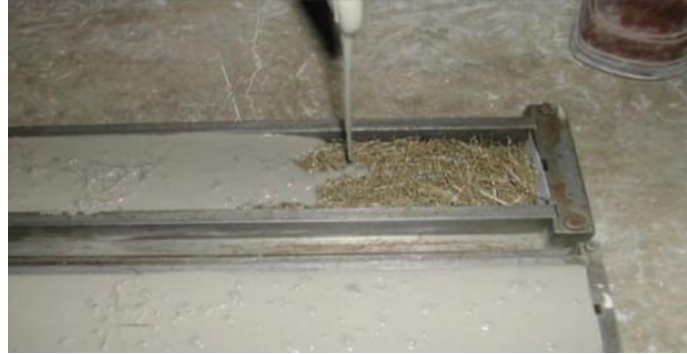
FIGURE 1. Casting procedure of SIFCON (Yazıcı, H., Yiğiter, H., Aydın, S., & Baradan 2006).
