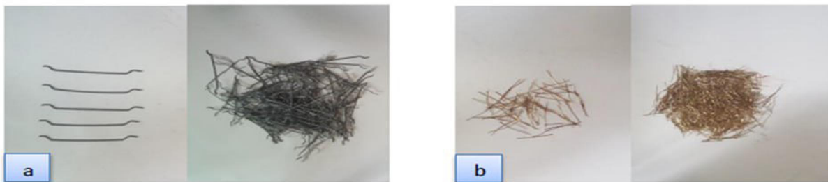
FIGURE 6. The steel fibers used: a) hooked end and, b) micro fiber (Manolia Abed AL-Wahab Ali 2018)
