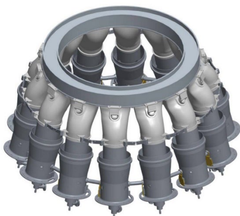
FIGURE 2. Combustor liner arrangement in gas turbine
